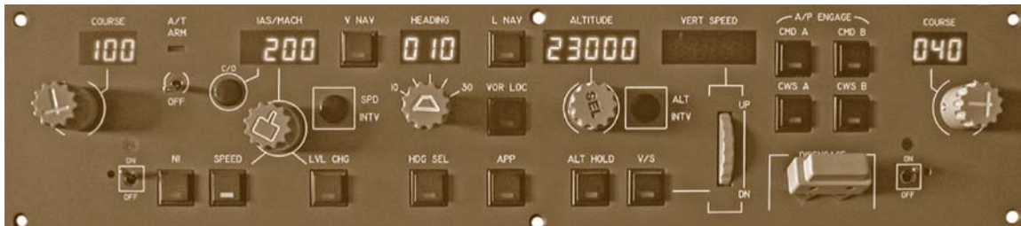
Fig. 68.4 Mode control panel (after [68.7])
