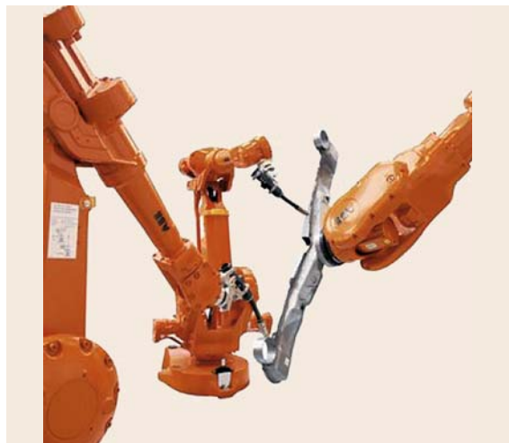
Fig. 32.10 The MultiMove function, which is embedded into the IRC5 software, allows up to four robots and their work-positioners or other devices to work in full coordination
