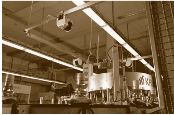
Fig. 39.2 Safety laser scanner application (courtesy of Sick Inc., Minneapolis)
