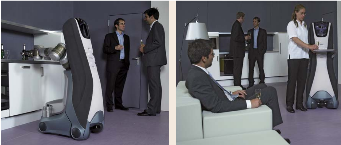
Fig. 84.14 Care-O-bot 3 fetching a drink in the kitchen and serving drinks to visitors
