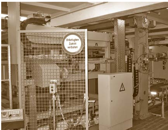
Fig. 34.17 Disjunctive safety device at a palletizing automaton
