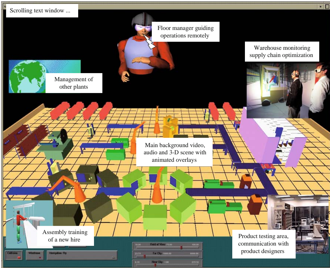
Fig. 15.2 Conceptual demonstration of remote facility management user interface showing many telecollaborative activities
