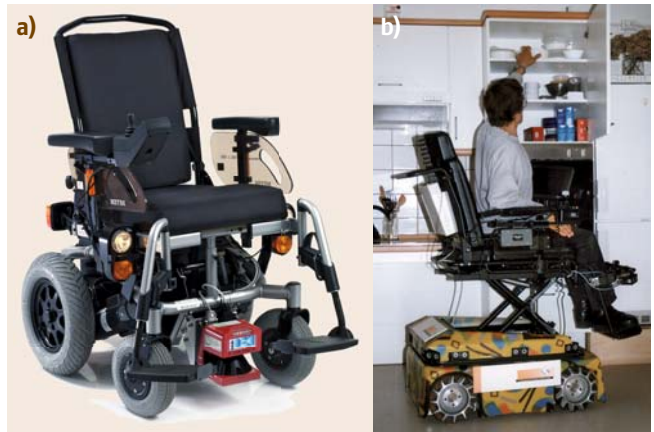
Fig. 84.4a,b Examples of advanced robotic wheelchairs: (a) Rolland III (courtesy of the DFKI-Labor, Bremen, Germany) and (b) OMNI (courtesy of Forschungsinstitut Technologie und Behinderdung der Evangelischen Stiftung Volmarstein, Germany)
