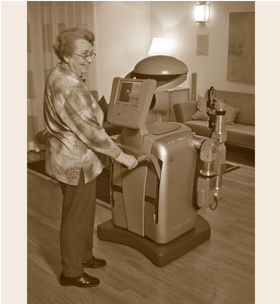
Fig. 34.19 Care-O-bot is a supporting system for the care of elderly people (photo taken with permission of Fraunhofer IPA)
