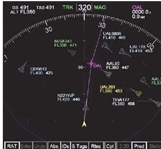
Fig. 68.7 NASA flight deck display of traffic information (after [68.21])
