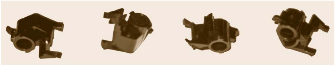
Fig. 50.5 Four of 12 stable states for a complex part
