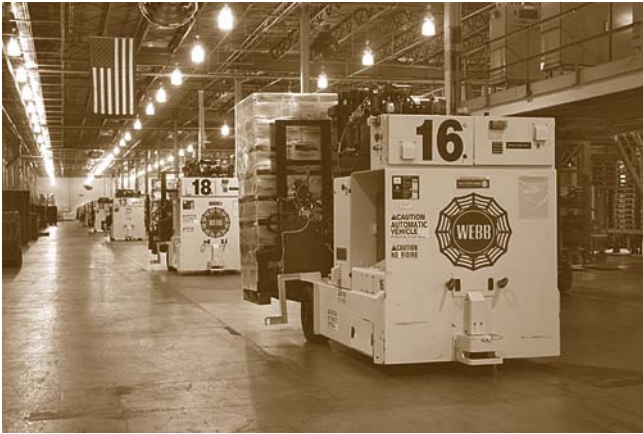
Fig. 54.2 Inertial guidance automatic guided vehicle (courtesy of the Jervis B. Webb Company)
