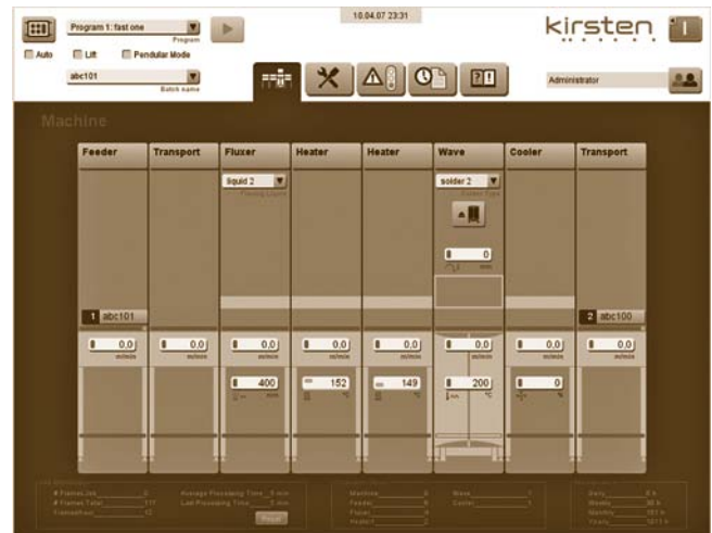
Fig. 23.4 The modularity of the machine is reflected on the graphical user interface
