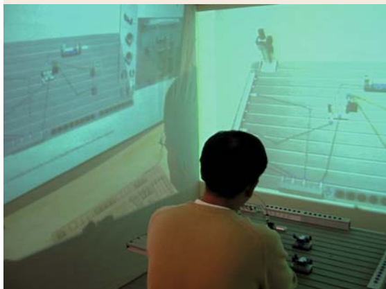
Fig. 41.11 Workspace with the real workbench and the virtual one in front, and the remote collaborators projected onto the left and right canvases
