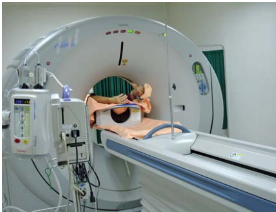
Fig. 80.5 A multislice CT volume scan system (photo courtesy of Cheng Ching General Hospital)
