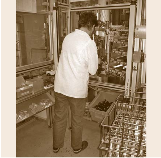
Fig. 34.18 Safety measure with approximation function (light barrier) at a partly automated assembly area
