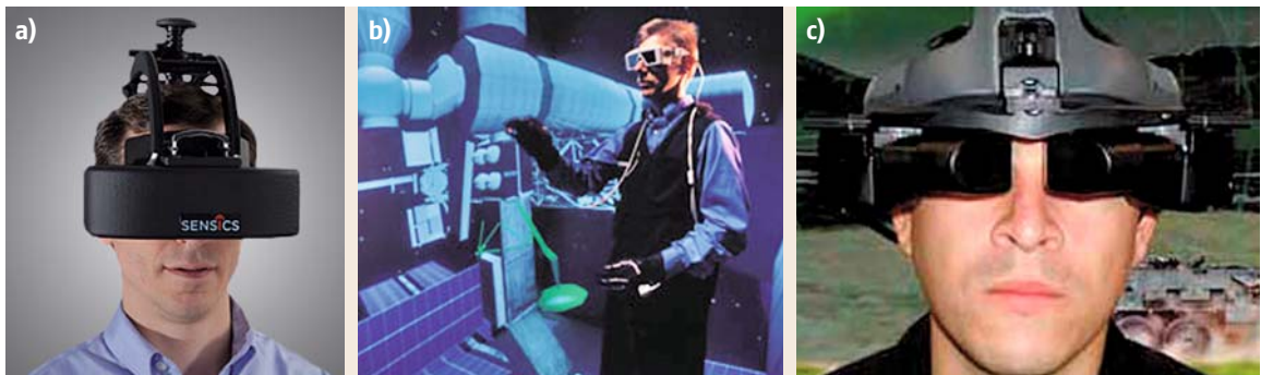
Fig. 15.1 (a) Sensics piSight head-mounted display for virtual prototyping, training, data mining, and other applications ( http://www.sensics.com/ , December 2007). (b) Pinch is an interacting system for interacting in a virtual environment using sensors in each fingertip ( http://www.fakespace.com/ , December 2007). (c) Proview SR80 full-color SXGA 3-D stereoscopic head-mounted display ( http://www.vrealities.com/ , December 2007)
