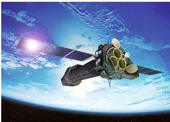
Fig. 69.1 The European Space Agency's (ESA) XMM-Newton is the most sensitive x-ray telescope ever built. Its high-technology design uses over 170 wafer-thin cylindrical mirrors spread over three telescopes. This unique x-ray observatory was launched by Ariane 5 from the European spaceport at Kourou in French Guiana on 10 December 1999 (courtesy of ESA)
