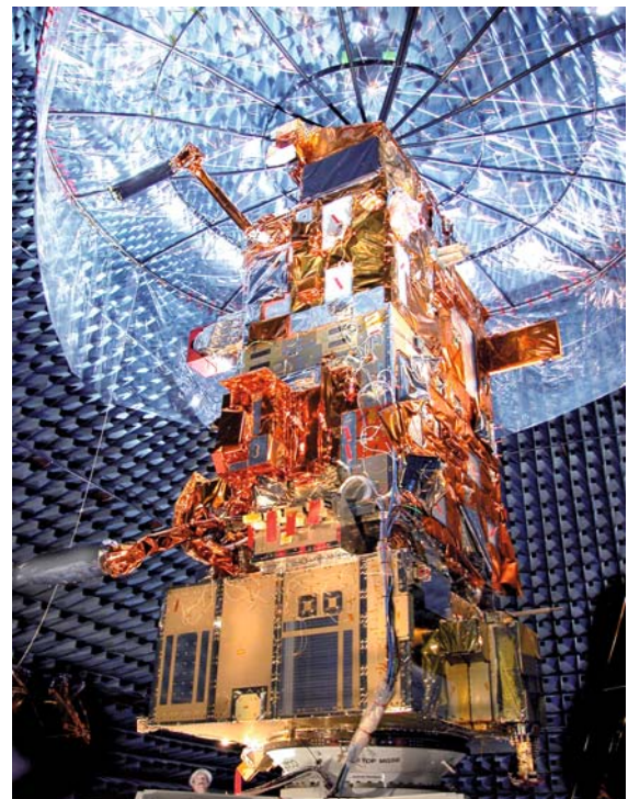
Fig. 69.10 MetOp-A satellite undergoing final testing at EADS Astrium's facilities in Toulouse. MetOp-A was launched on 19 October 2006 from the Baikonur Cosmodrome in Kazakhstan, on a Soyuz ST rocket with a Fregat upper stage (courtesy of ESA)
