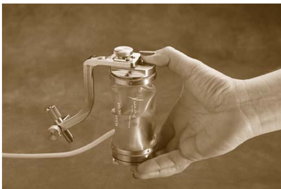
Fig. 78.2 Mazor's SpineAssist miniature robot for spine surgery
