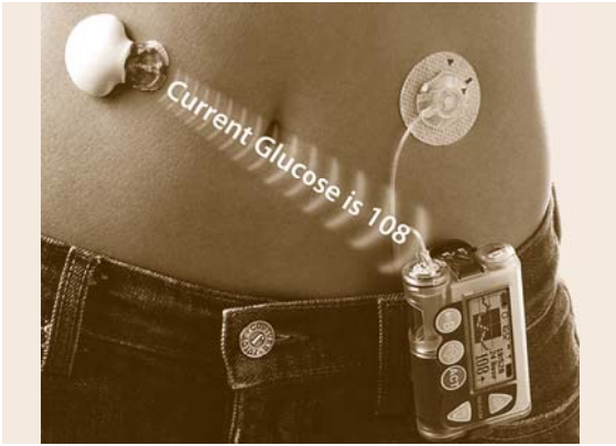
Fig. 76.7 Diabetic patient using a wireless subcutaneous glucose sensor communicating the measurement to the data storage device. This device also includes the insulin pump mechanism; note that the pump is not altering insulin delivery rate based on the glucose measurement unless commanded to do so by the patient (courtesy of Dr. Cesar Palerm, Medtronic Diabetes)
