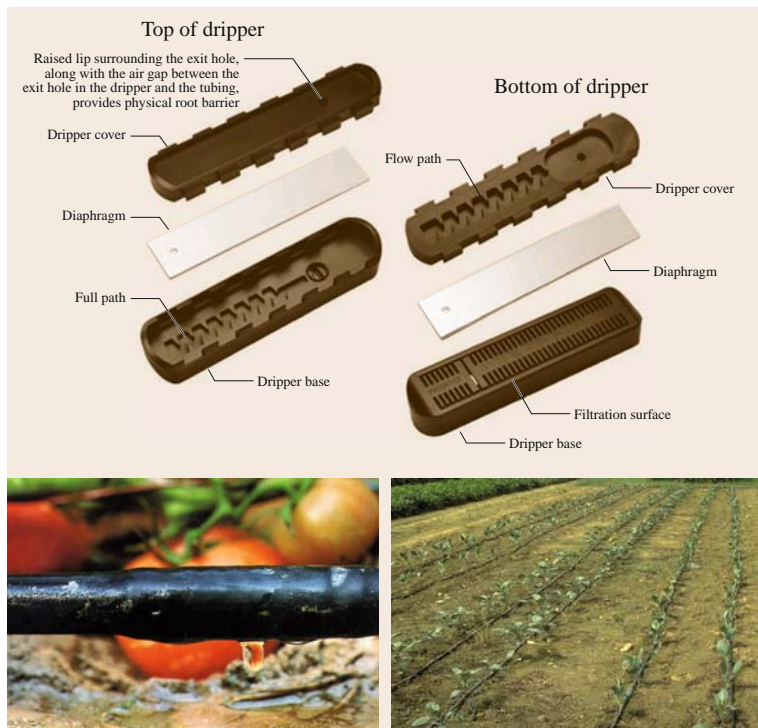
Fig. 63.7 Dripper and drip line irrigation system (courtesy of Netafim)
