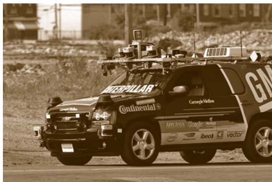
Fig. 66.8 Carnegie Mellon entry to the DARPA 2007 Urban Challenge competition, Boss, Tartan racing robot (courtesy of Tartan Racing, Carnegie Mellon University)
