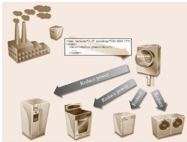
Fig. 83.12 Direct load control using smart power meters
