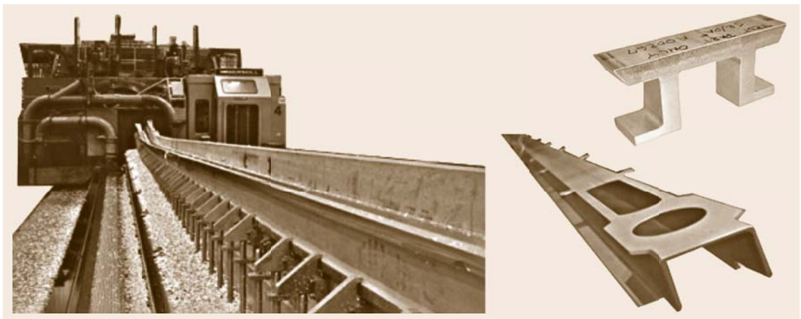
Fig. 51.3 Dedicated spar mill gantry with typical cross section and machined part
