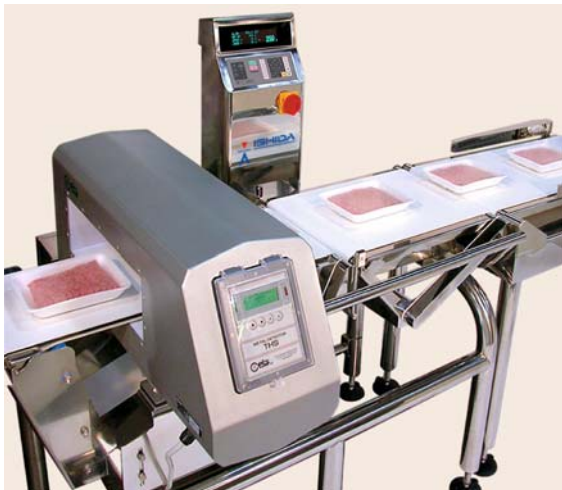
Fig. 60.6 Combined check weight and metal detection station
