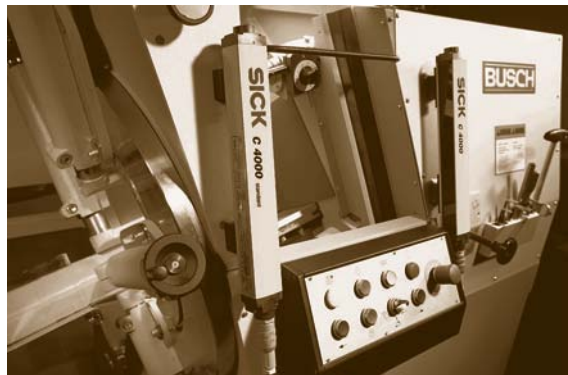
Fig. 39.3 C4000 safety light curtain hazardous point protection (courtesy of Sick Inc., Minneapolis)
