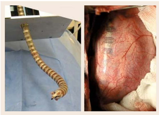
Fig. 78.10 CardioArm – a hyper redundant snake like robot for cardiac surgery
