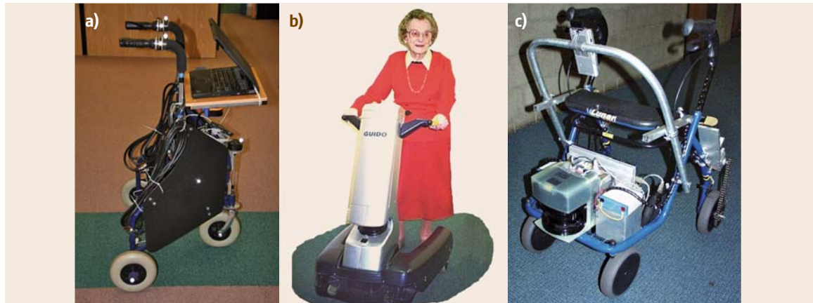
Fig. 84.2a–c Examples of passive robotic walkers: (a) COOL Aide (courtesy of the University of Virginia, USA), (b) Guido (courtesy of Haptica Ltd., Dublin, Ireland), and (c) CMU robotically augmented walker (courtesy of Carnegie Mellon University, Pittsburgh, USA)
