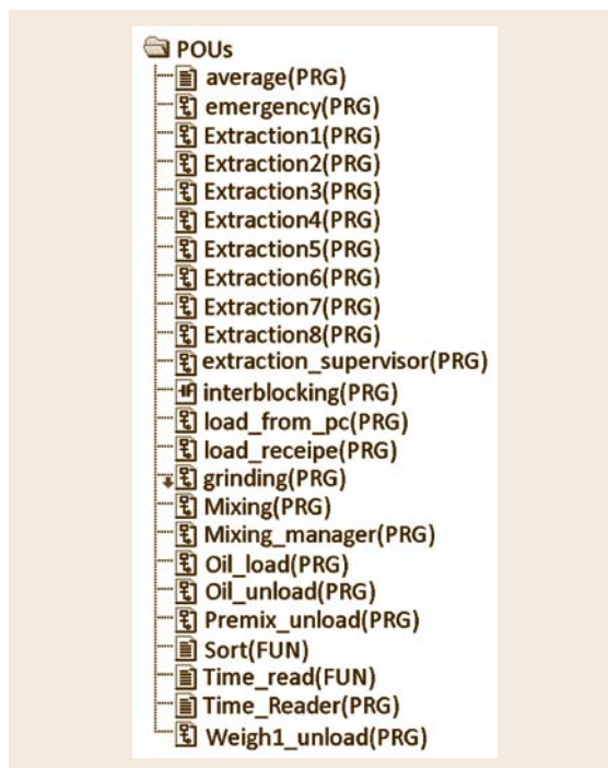
Fig. 64.3 Structure of the software project
