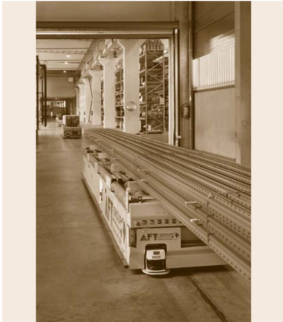
Fig. 39.4 Safety laser scanner AGV (automated guided vehicle) application (courtesy of Sick Inc., Minneapolis)
