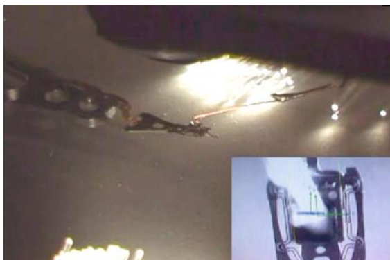
Fig. 50.9 Visual servoing: steering parts into alignment using vision in motion control loop (courtesy of Precise Automation)
