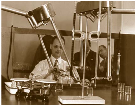
Fig. 27.1 Raymond Goertz with the first mechanically coupled teleoperator (Source: Argonne National Labs)
