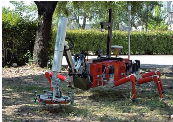
Fig. 27.14 SILO6: A six-legged robot for humanitarian demining tasks (courtesy of IAI, Spanish Council for Scientific Research – CSIC)
