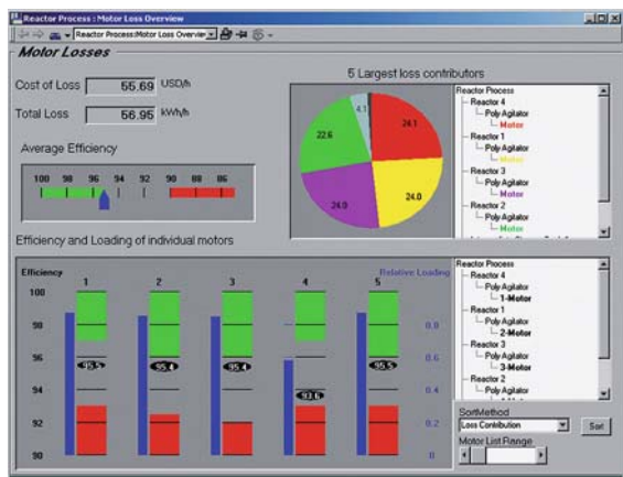
Fig. 33.4 Real-time measurement of the energy efficiency of five motors in a plant [33.7]
