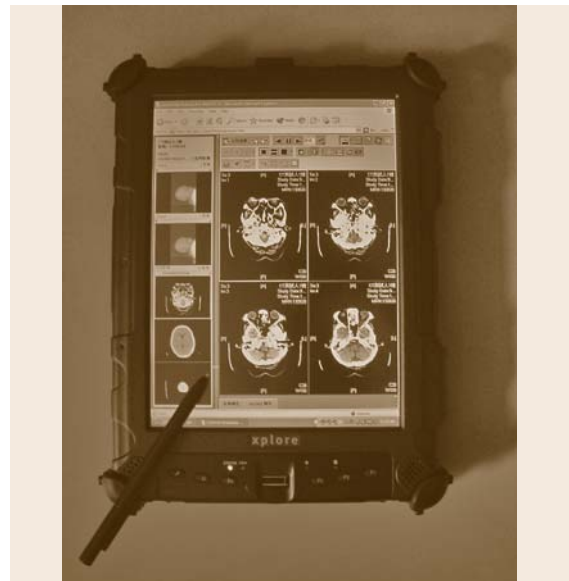
Fig. 80.3 Portable medical order-entry device (photo courtesy of DVNET Technology Co., www.dvnet.biz )
