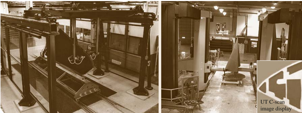
Fig. 51.17 Two types of automated ultrasonic inspection systems: independent tower system ( right ) and gantry system ( left ) (courtesy of Boeing)
