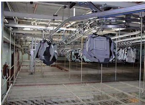
Fig. 16.1 Car seat covers industrial automated warehouse system based on overhead trolleys [16.1]
