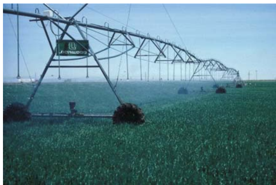
Fig. 63.6 Center pivot with drop sprinklers (courtesy of Conversation and Production Res. Lab., Bushland, TX, USDA, ARS)
