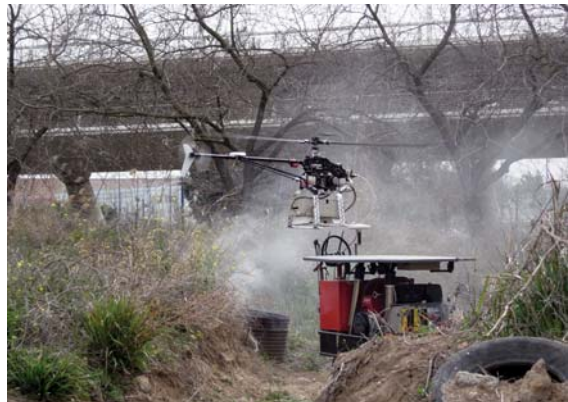
Fig. 16.15 Experiment of the CROMAT system for the cooperation of aerial and ground robots [16.53], http://grvc.us.es/cromat
