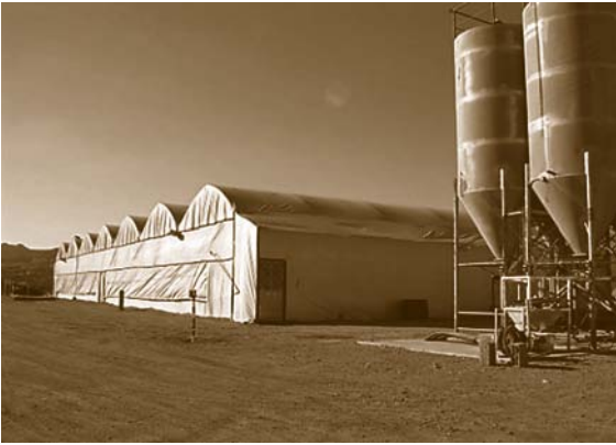
Fig. 63.18 Aquaculture closed system with a feeding station. Feed quantities are calculated on a daily basis to each fish tank according to fish weight, water temperature, and growth rate
