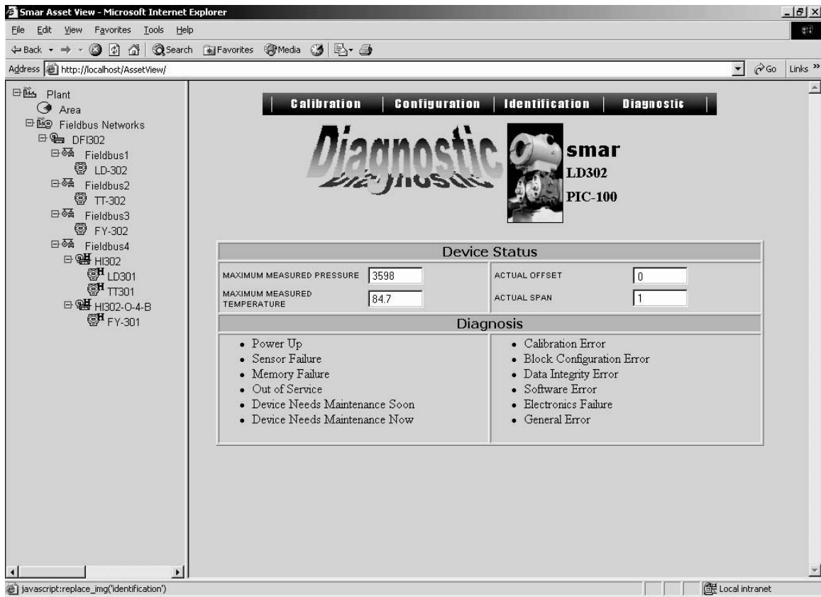
FIG. 3.9n Transmitter diagnostics using Web-based asset management (OPAM) software.
