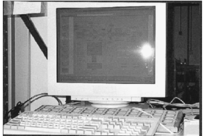
FIG. 4.24e A workstation with an alarm annunciator panel and keyboard.
