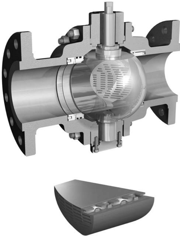
FIG. 6.16p Multistage low-flow control valve design with anticavitation and antinoise capability. (Courtesy of Control Components Inc.)
