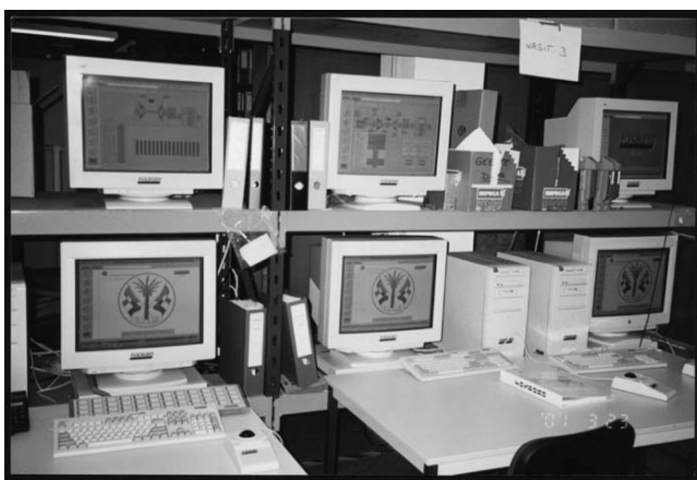
FIG. 4.24d An intelligent workstation-based DCS.
