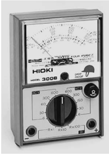
FIG. 1.1h An analog multimeter. (Courtesy of Hioki Corporation, www.hioki-usa.com .)
