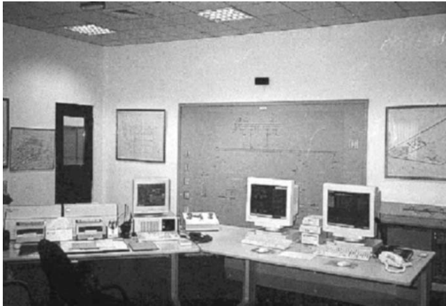
FIG. 4.24c A diskless workstation-based DCS.
