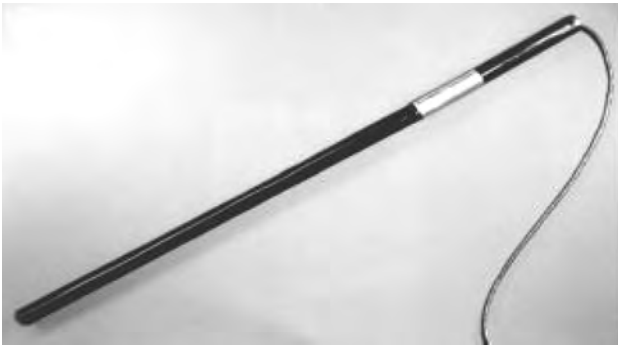
FIG. 8.34k Dielectric constant monitoring probe for the remote measurement of soil moisture. (Courtesy of Automata Inc.)
